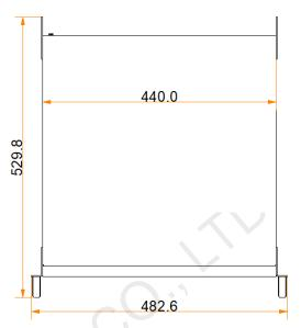
Tolerance: ±0.3 Unit: mm
