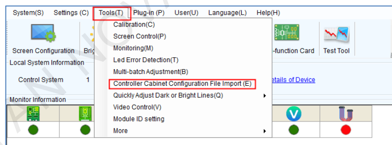
Figure 5-4 Importing controller cabinet configuration files
